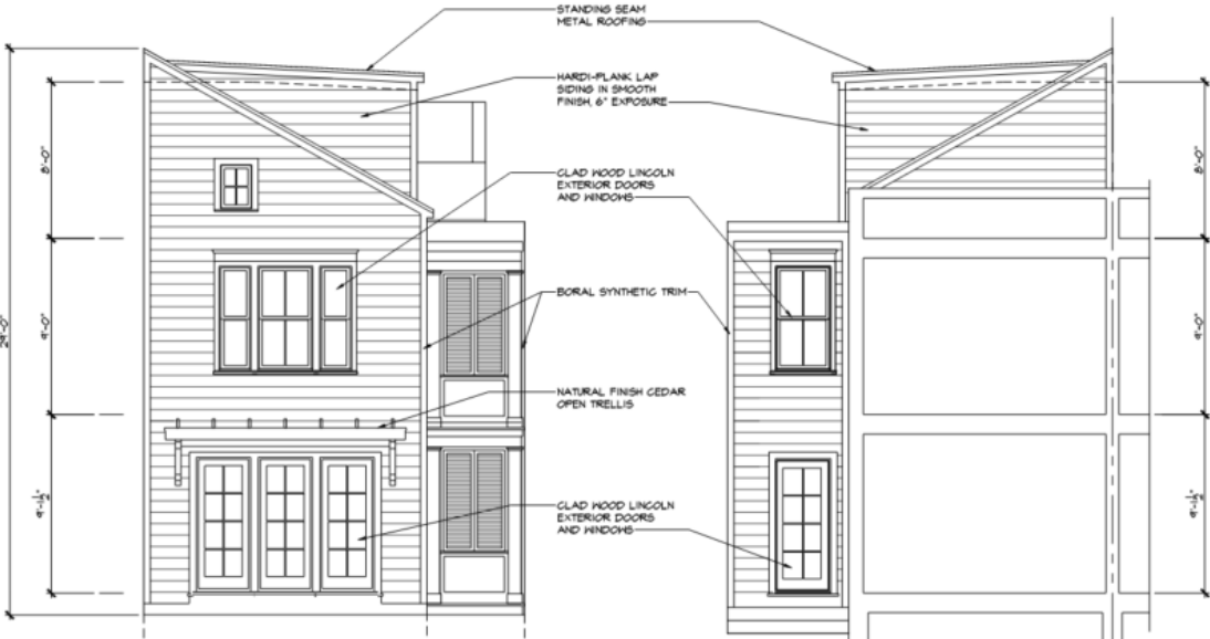
Figure 3: East elevation and section of proposed addition
