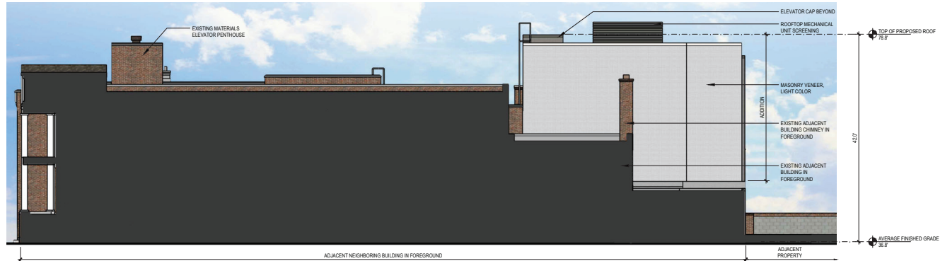
2 EAST BUILDING ELEVATION (PROPOSED) A5 SCALE: 1/8" = 1'-0"
