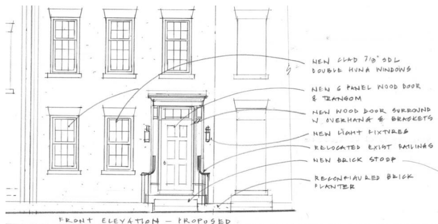
Figure 2: Proposed primary elevation
