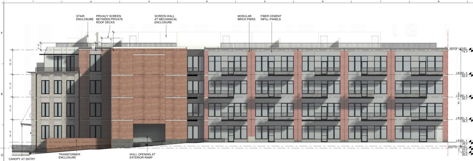
1 COURTYARD ELEVATION (DSUP) 1/8" = 1'-0"
