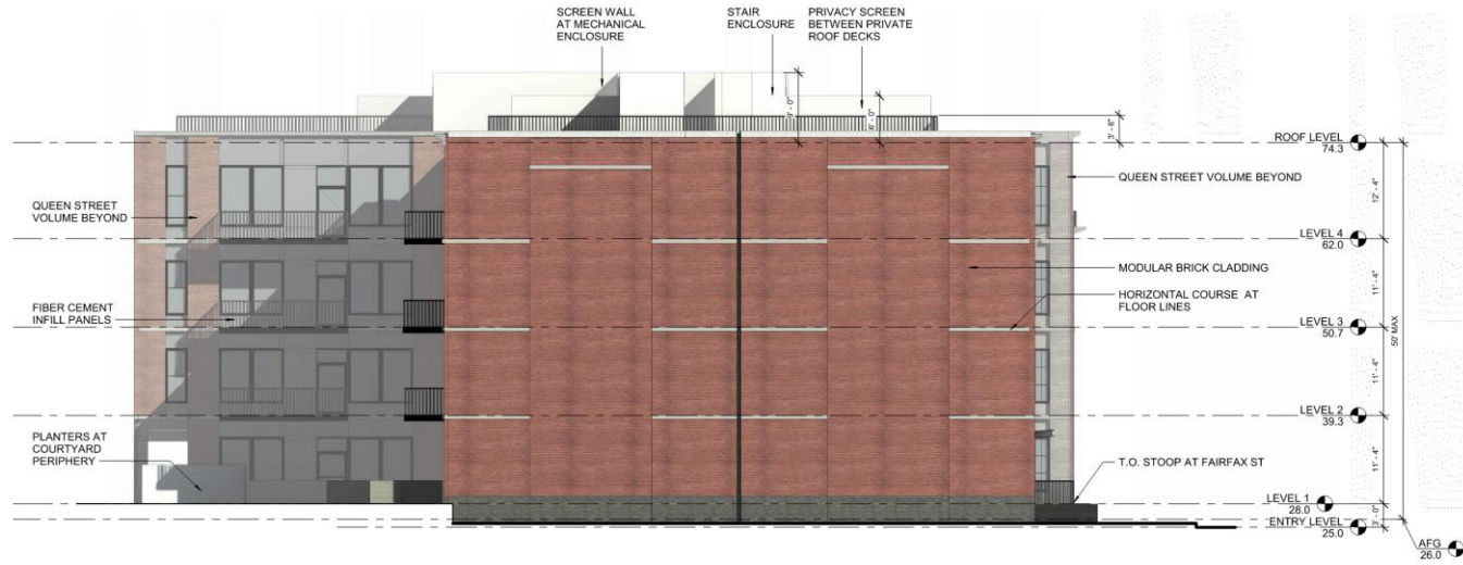
1 NORTH ELEVATION (DSUP) 1/8" = 1'-0"
