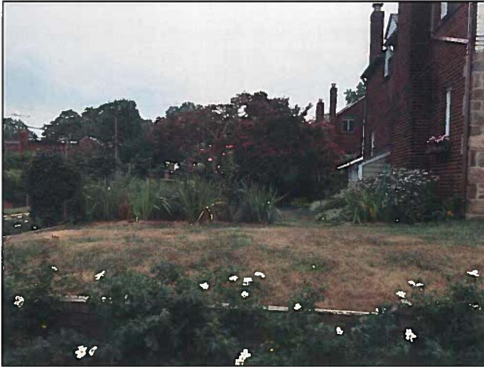
This is the current front yard at 800 Devon Place, Alexandria, VA 22314. The fence that was here fell down in the spring. The posts were not footed into concrete so the fence posts shifted and the slats fell down. The replacement fence will be made of cedar and footed in concrete.
