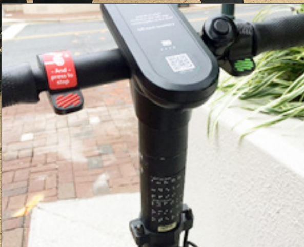
Braille messaging on a scooter for identification by people with vision disabilities
