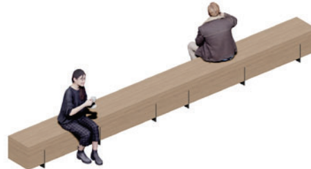
Wood Block Bench w/ Metal Support @ Seating Nooks BENCH TYPE -02A (SF-20)
