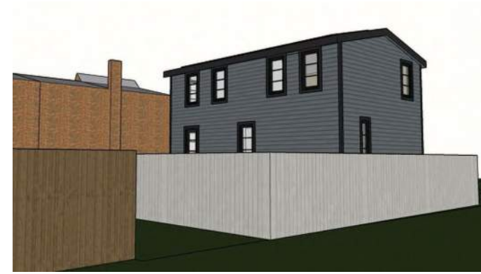
South Facade (rear) 1. ADU removed 2. Windows resized to match adjacent homes and increase privacy between homes
