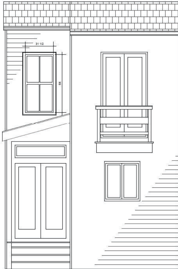
EXISTING EXTERIOR REAR ELEVATION
