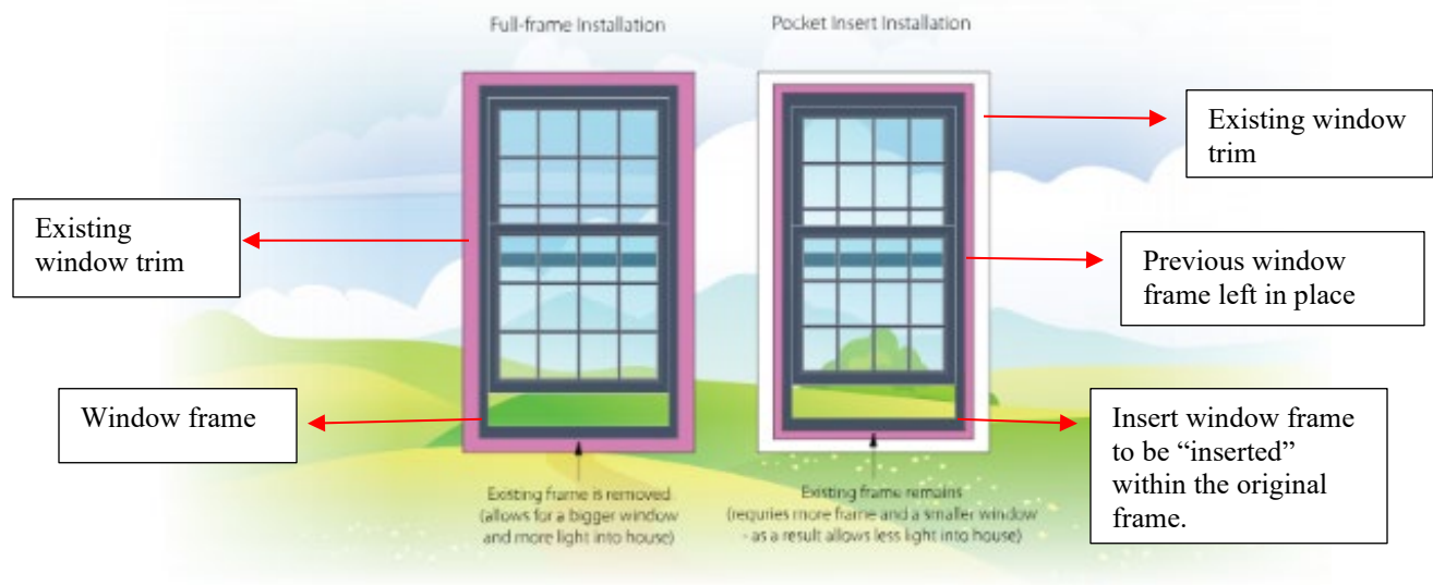
Figure 3: Insert vs. full frame windows
