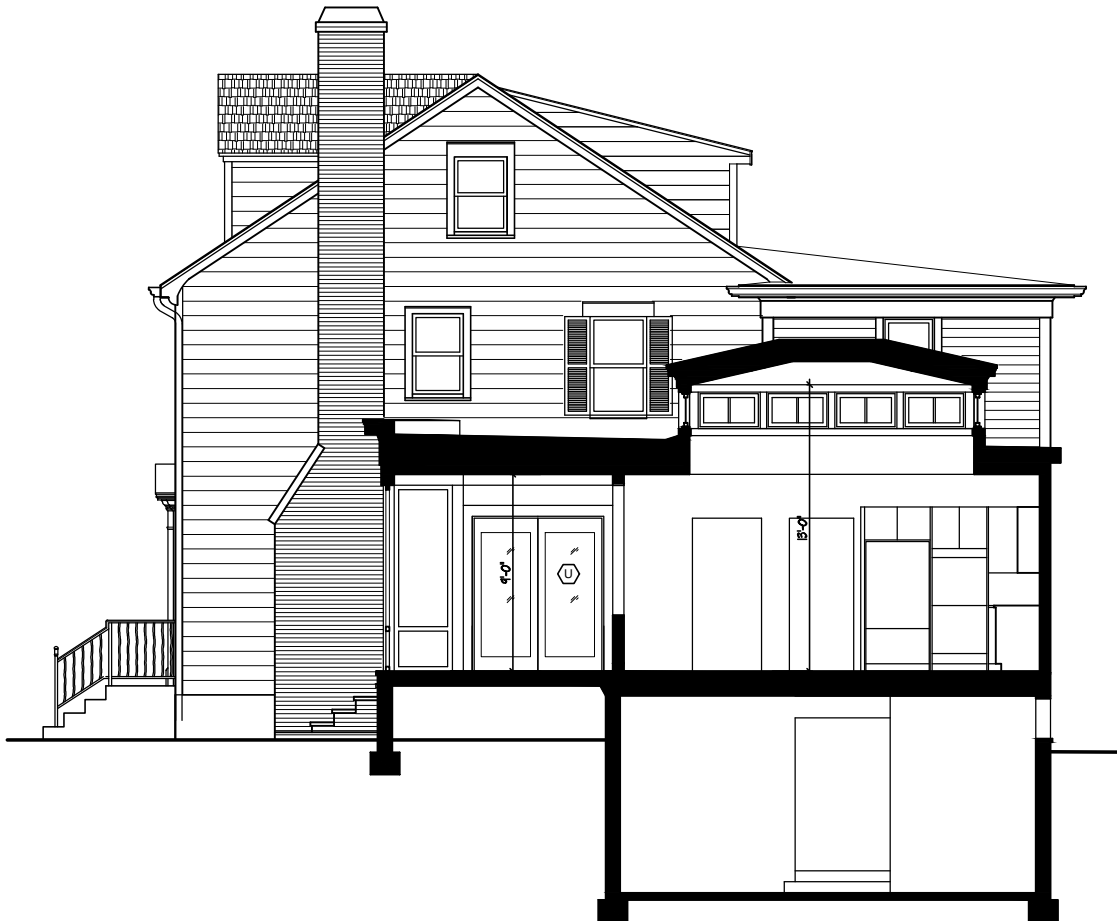
1 SECTION - KITCHEN, DINING & SCREEN PORCH A-4.0 SCALE: 1/4" = 1'-0"
