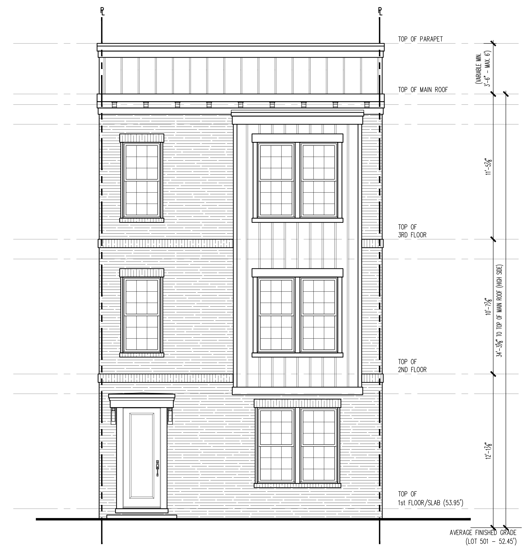
FRONT ELEVATION (LOT 501) SCALE: 1/4" = 1'-0"
