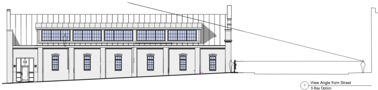
Figure 3: View of N Fairfax Street façade and site section showing visibility of dormer
