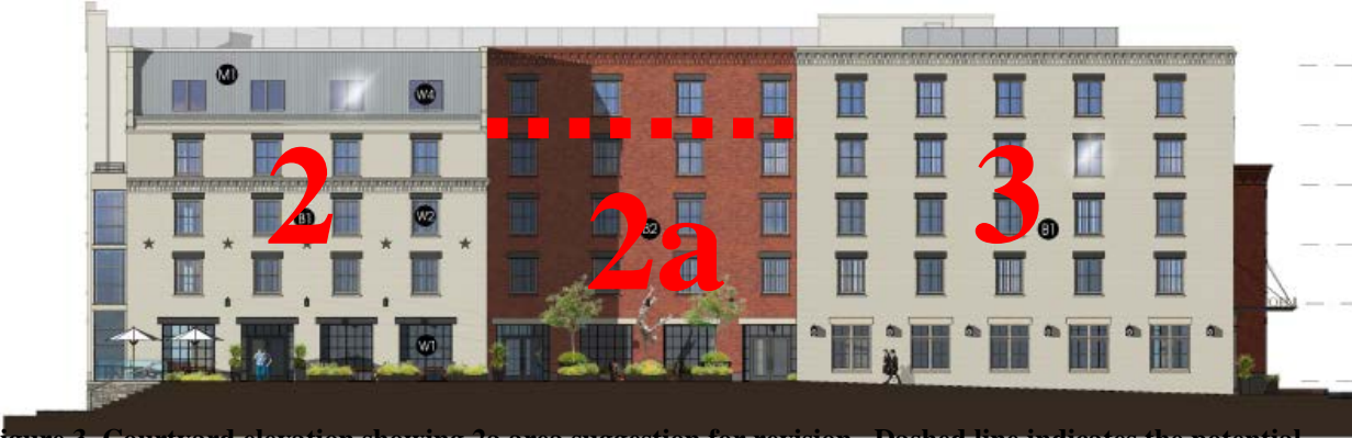
Figure 3. Courtyard elevation showing 2a area suggestion for revision. Dashed line indicates the potential continuation of pitched roof with lighter building 2 color.
