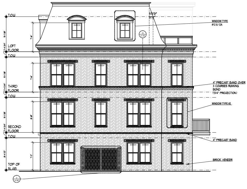
1 Unit B - Side Elevation #5 Scale: 1/4" = 1'-0" Building #3 Lots: 111
