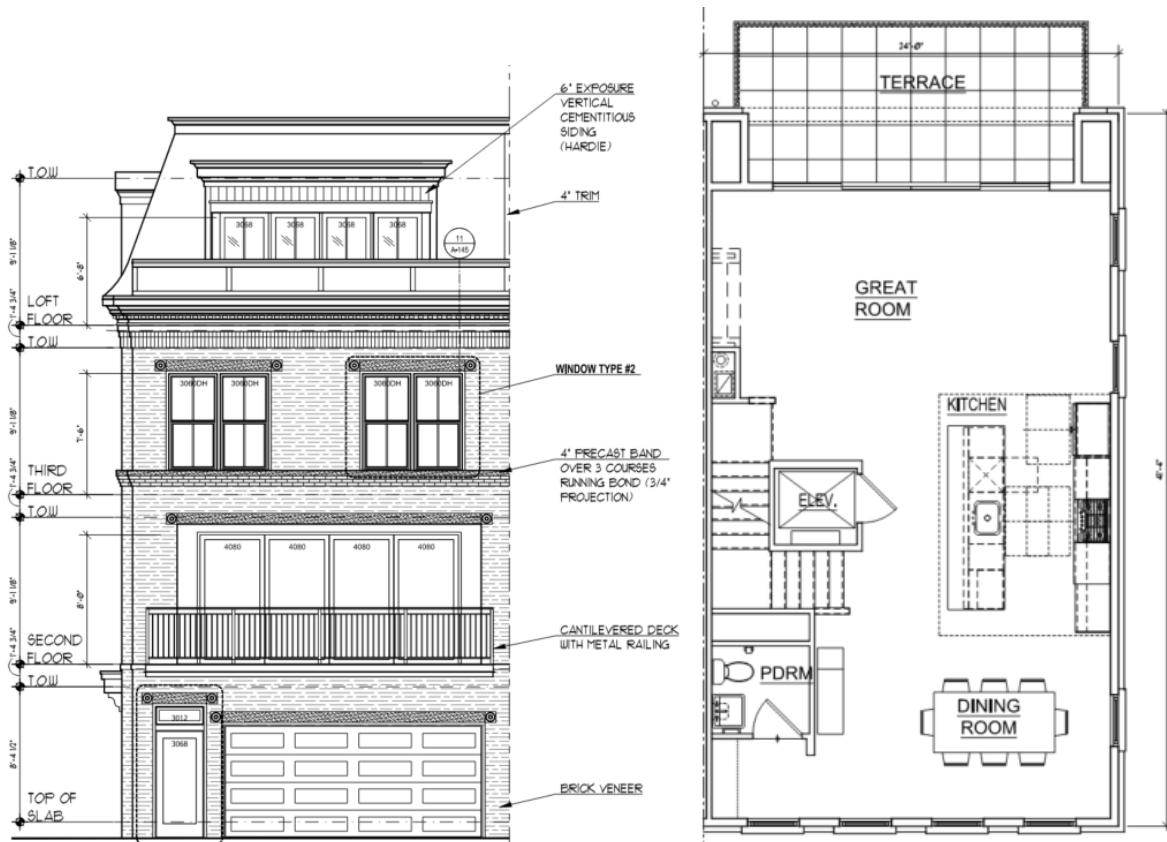
Figure 10: Elevation and plan showing recessed area at rear terrace
