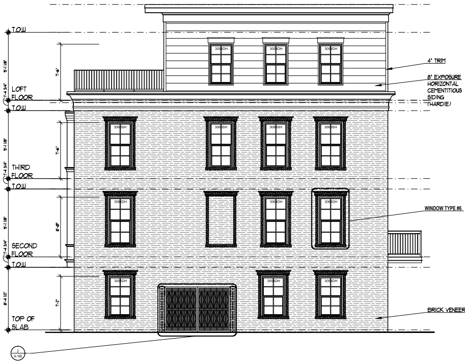
2 Unit C - Side Elevation #4 Scale: 1/4" = 1'-0" Building #6 Lots: 125
