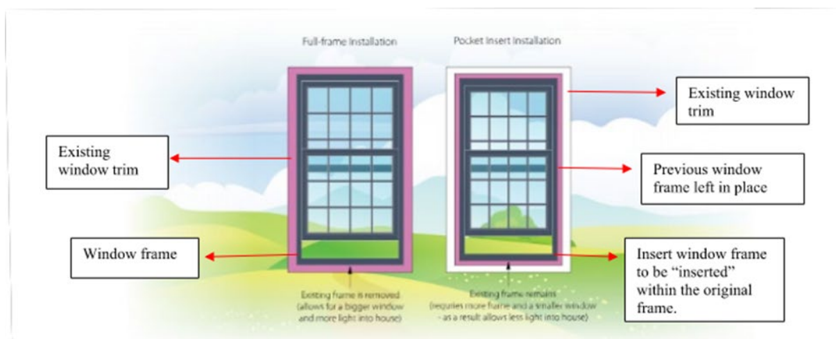
Figure 1: Insert vs. full frame window
