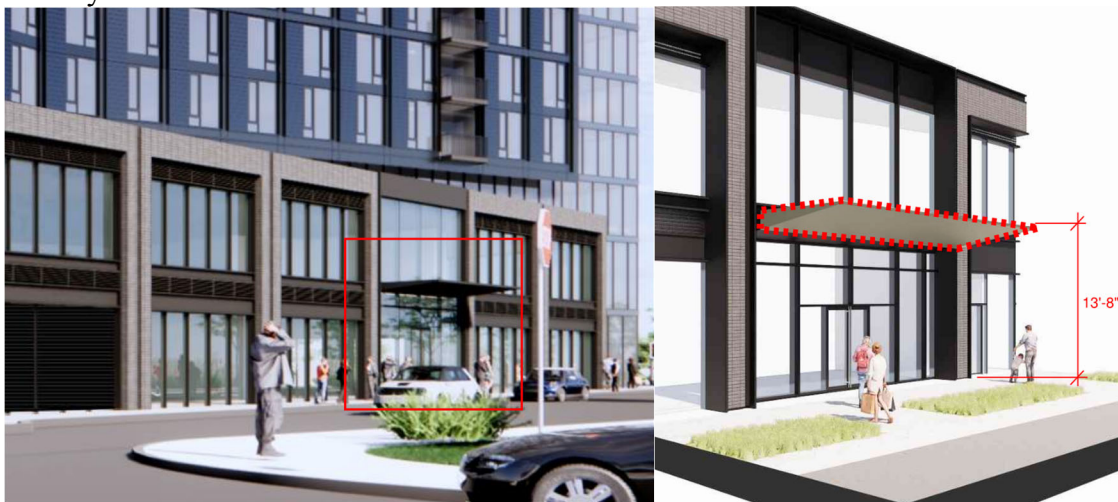
Figure 17: Location of encroaching entrance canopy along Road A facade.
