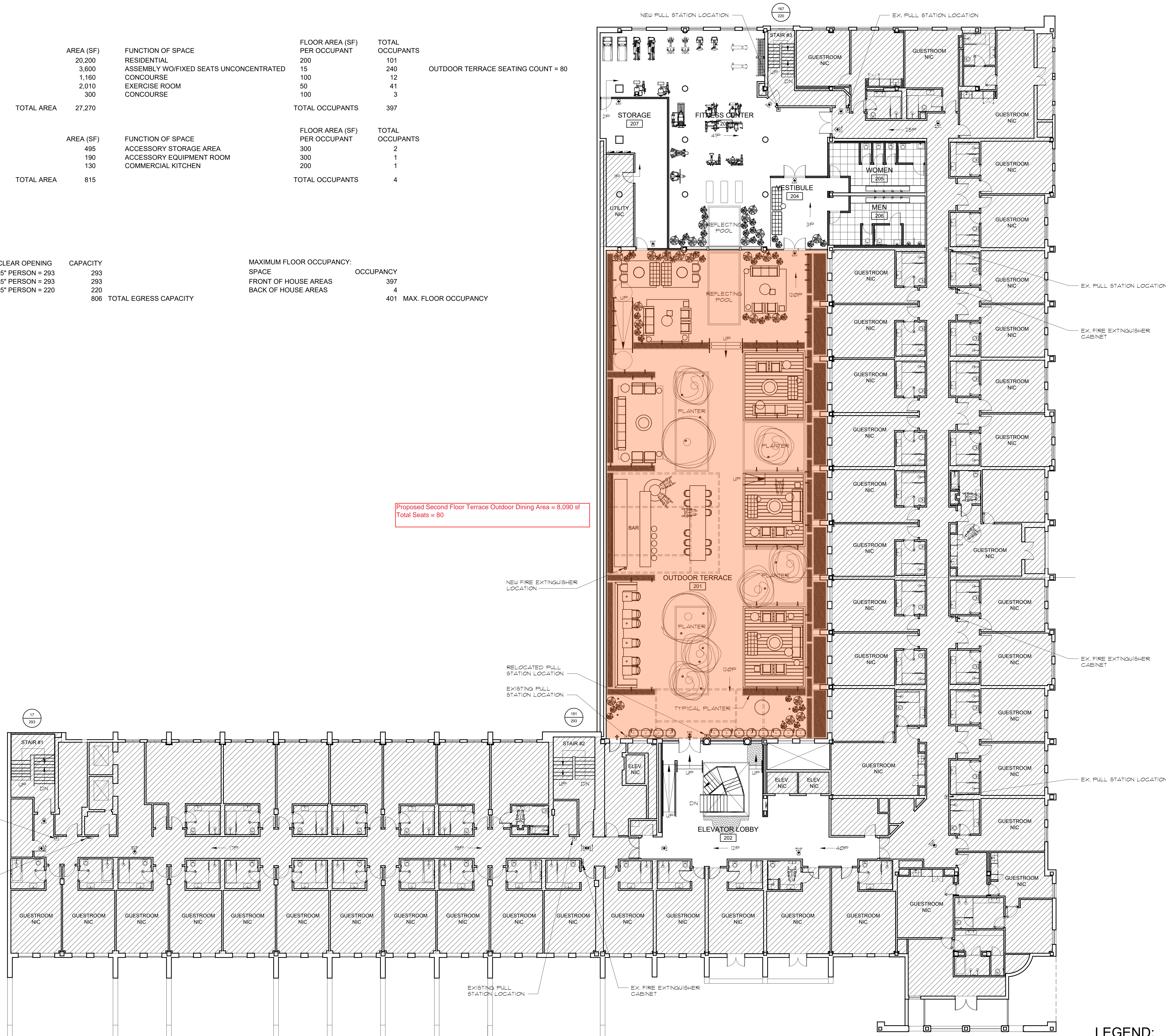
1 SECOND FLOOR EGRESS PLAN SCALE: 3/32"=1'-0"
