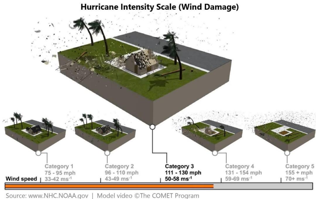
**Figure 44: Potential Wind Damage to Building in Major Category 3 Hurricane<sup>146</sup>**
