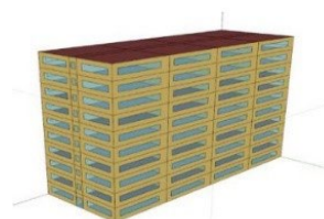
Figure 3. PNNL Highrise Multifamily Prototype
