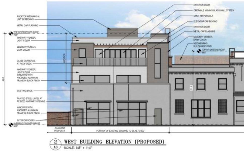
Figure 2: Proposed west elevation of addition
