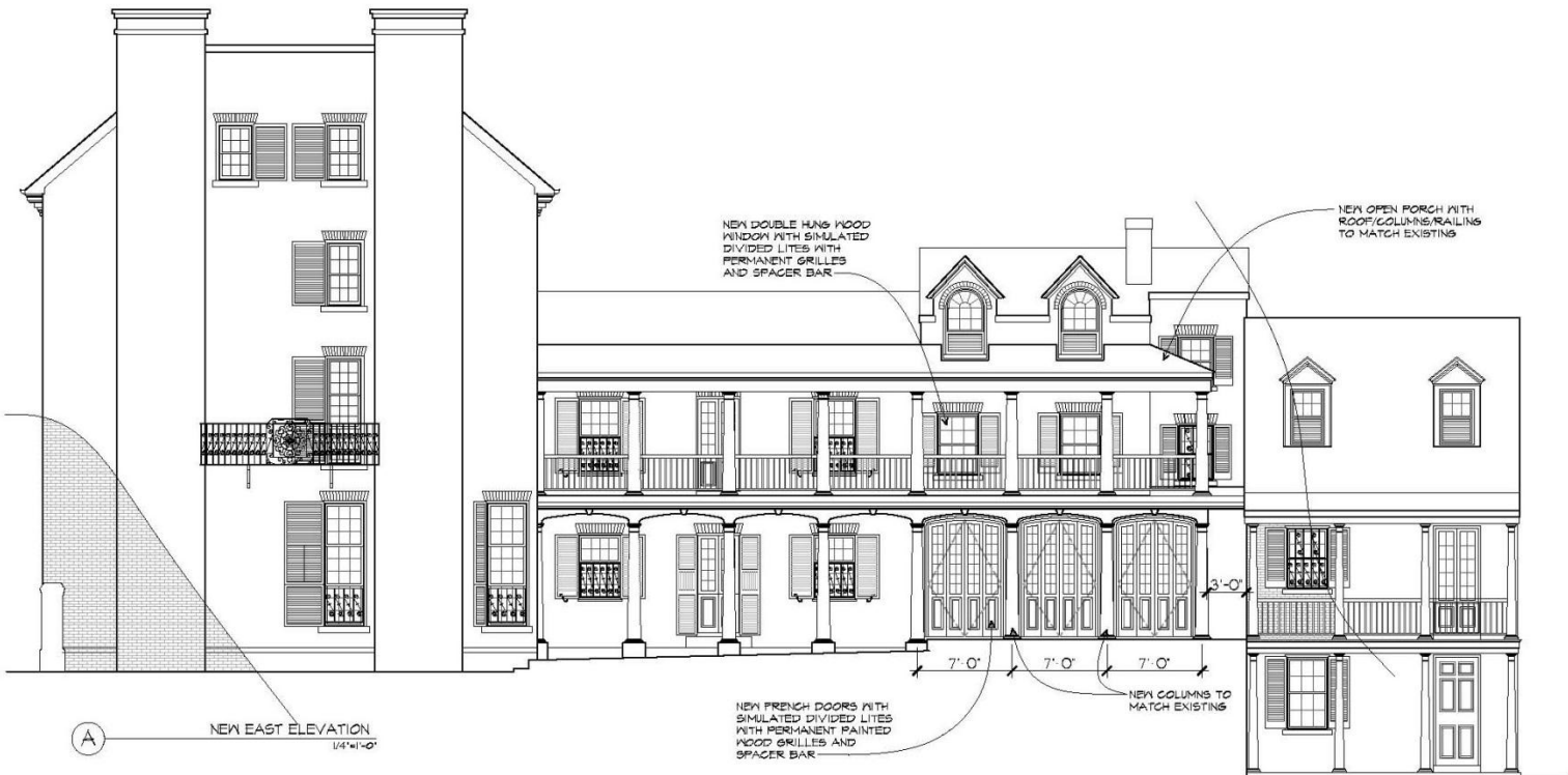
Figure 8: Initial proposal for east elevation, as submitted by applicant in March 2013. Note that the proposed replication and northern extension of the mid-20 th century, two story open porch obscures the original kitchen ell of the house. In this scheme, the modern porch becomes the dominant design feature. The north end of the porch also ends awkwardly in the middle of the hyphen windows.
