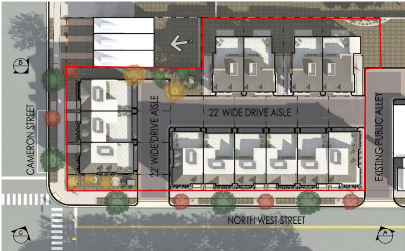
Figure 1: Illustrative site plan (townhouses face N. West and Cameron streets; semi-detached face private alley)
