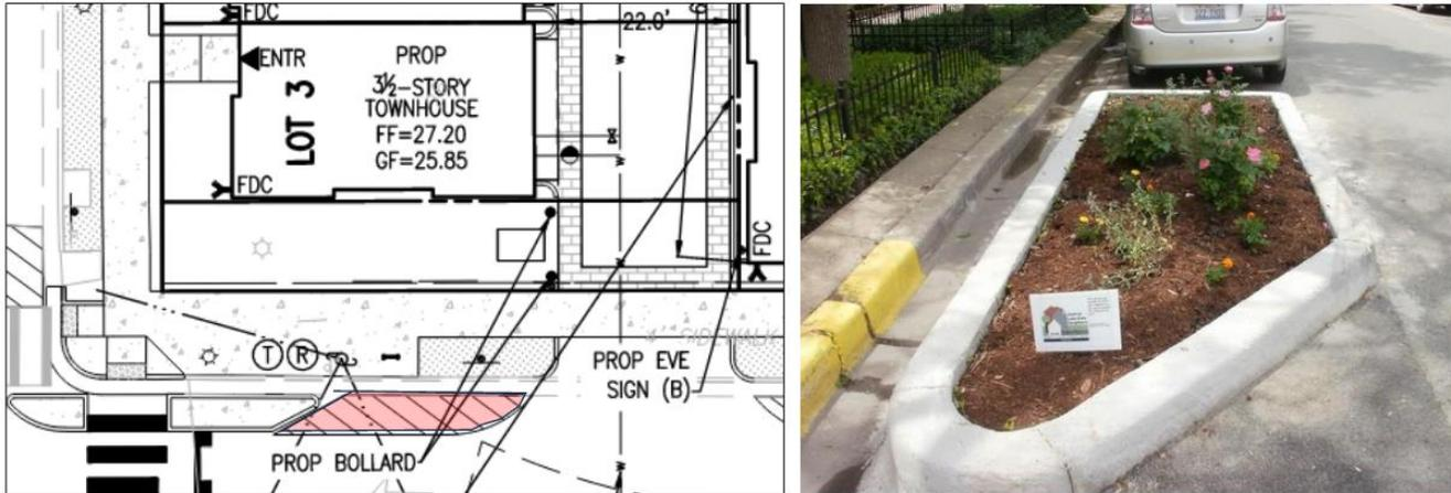
Figure 2: Area of pavement to be converted to curb extension with landscaping
