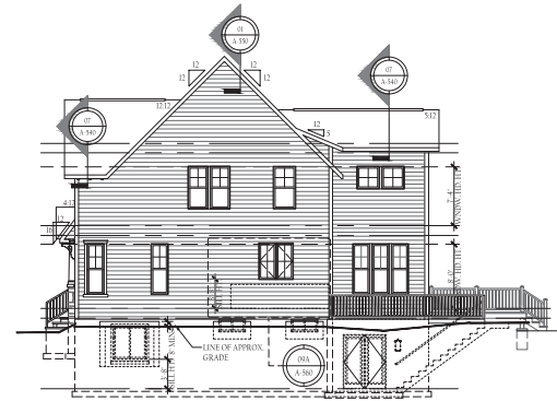
04 RIGHT SIDE ELEVATION SCALE: 1/4" = 1'-0"
