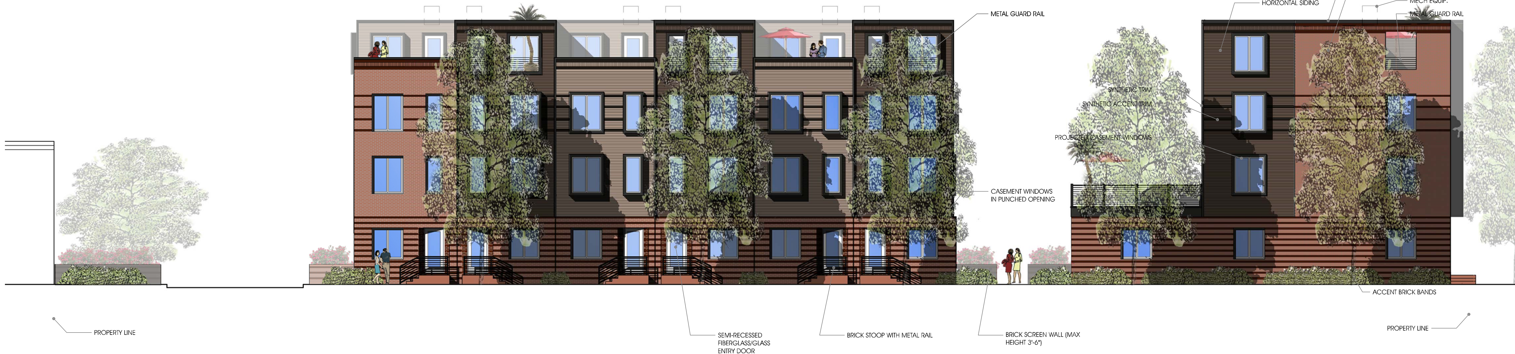
STICK #1 & #2 - WEST ELEVATION (FACING NORTH HENRY STREET) 1/8"=1'-0"
