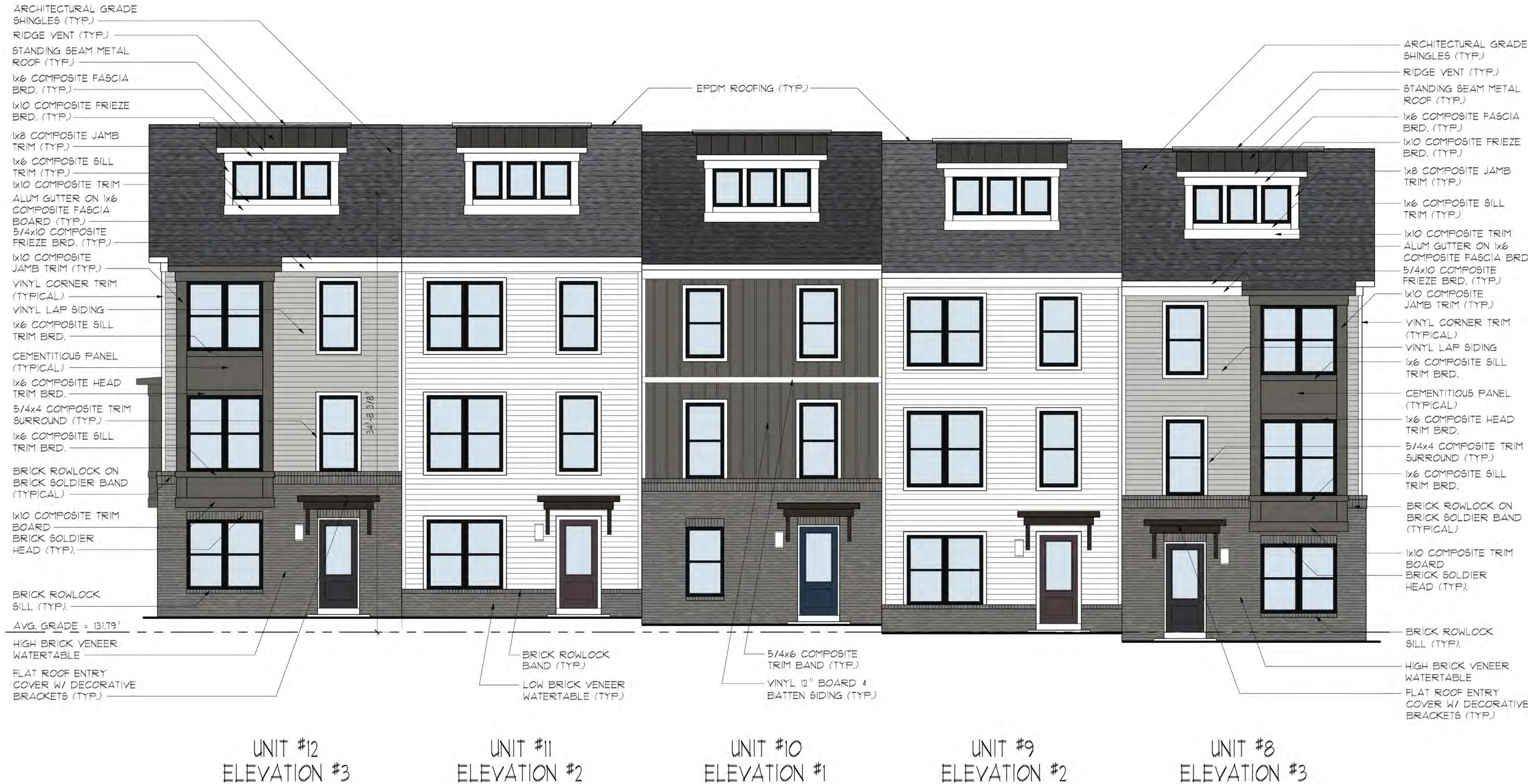
FRONT STRIP ELEVATION (UNIT #8 - #12)
