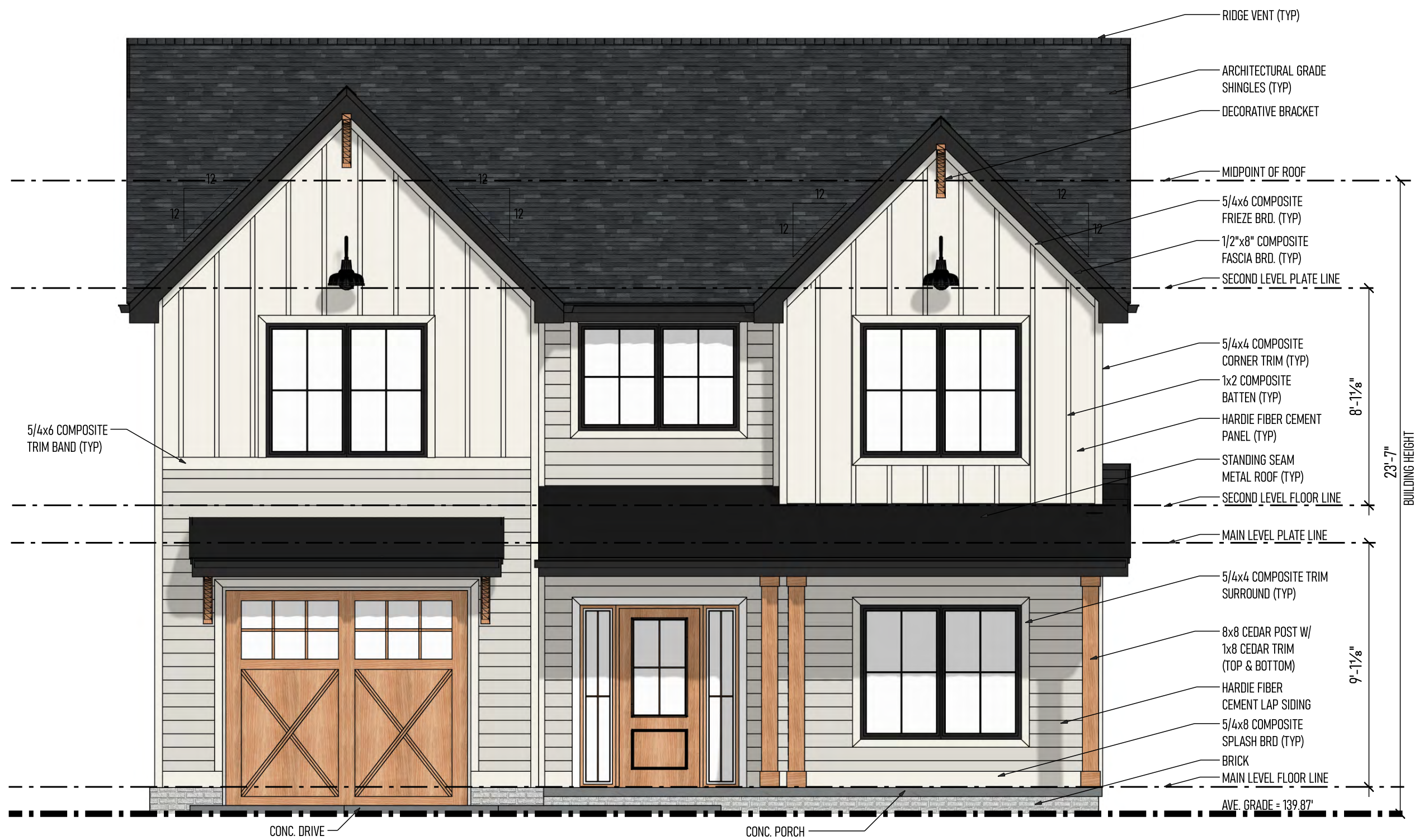
FRONT ELEVATION SCALE: 1/4" = 1'-0"
