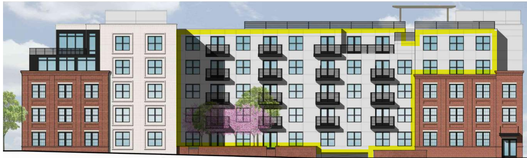
THE FIBER-CEMENT PANELS SHOWN ARE THE SAME AS THOSE APPROVED BY THE BAR FOR PORTIONS OF THE ALLEY FACADE OF THE ADJACENT "WHITLEY" CONDOMINIUM, 805-823 N. COLUMBUS STREET (CURRENTLY UNDER CONSTRUCTION).
