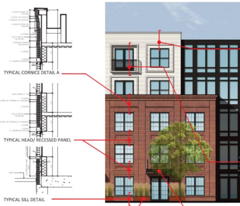
Figure 7: Masonry detailing at upper and lower portions of the proposed building
