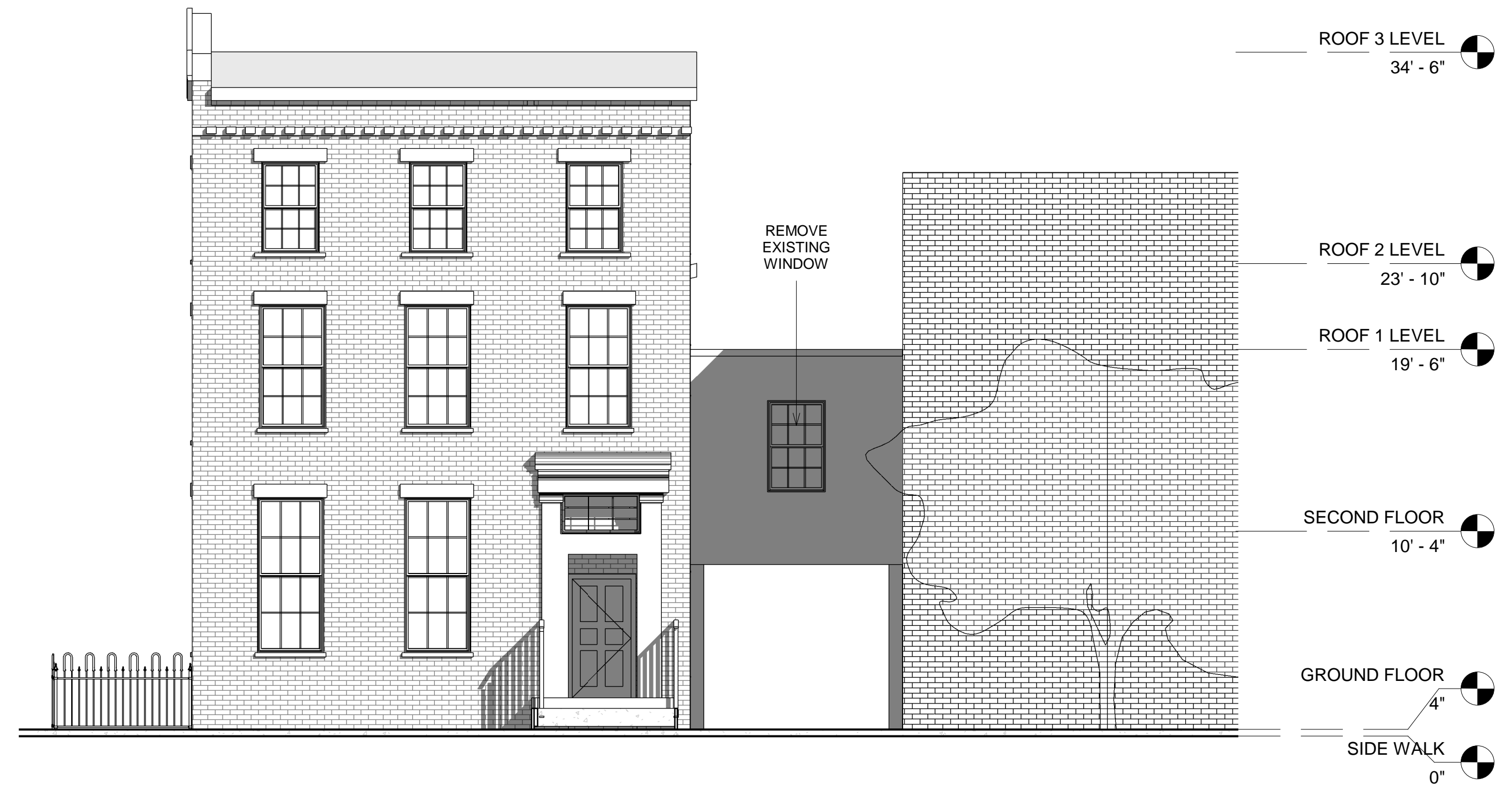
3 SOUTH ELEVATION @ PRINCE ST. 3/16" = 1'-0"
