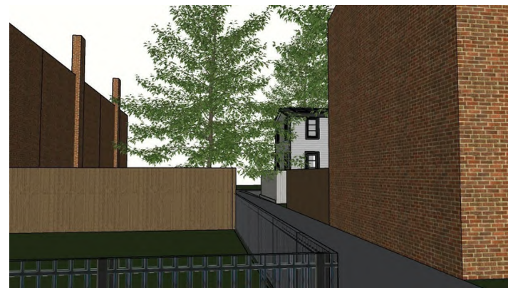
West Facade (side) 1. ADU removed 2. Windows resized to match adjacent homes and increase privacy between homes 3. Materials and colors modified to blend in with the neighborhood
