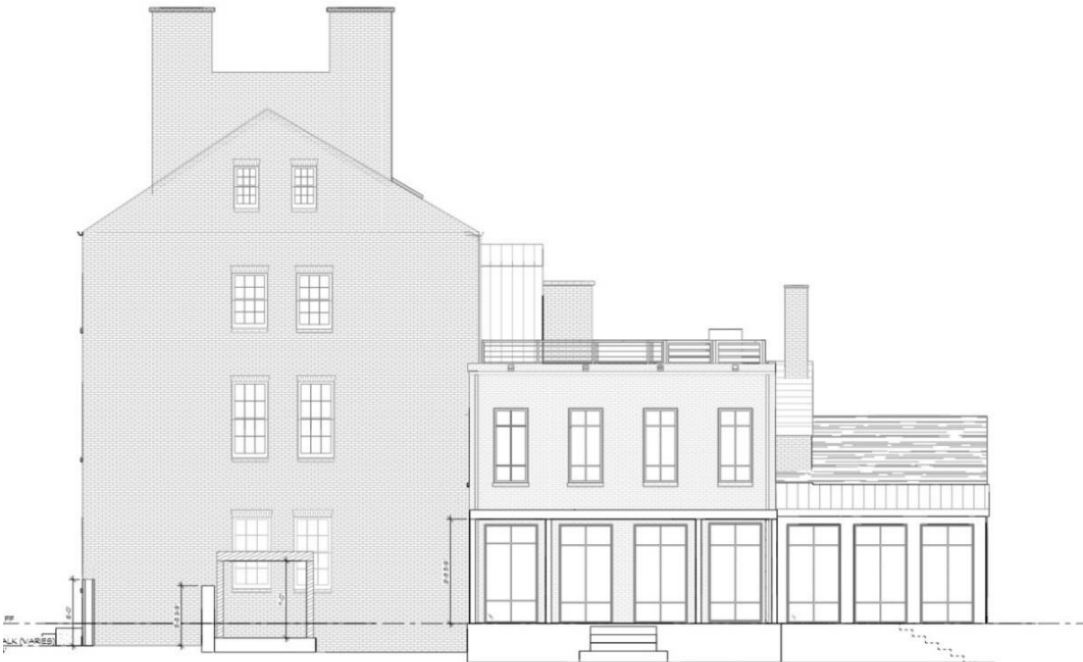
Figure 4: Current proposed south elevation; note that the support columns of the attached pergola now correspond to the window openings, giving a more balanced appearance.
