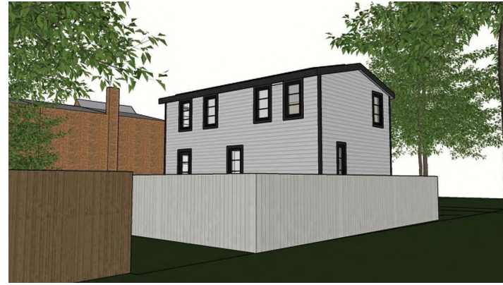
South Facade (rear) 1. ADU removed 2. Windows resized to match adjacent homes and increase privacy between homes 3. Materials and colors modified to blend in with the neighborhood
