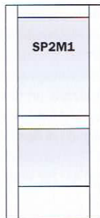
4 1/8" Stiles & Top Rail 5 1/8" Mid-Rail 12" Bottom Rail
