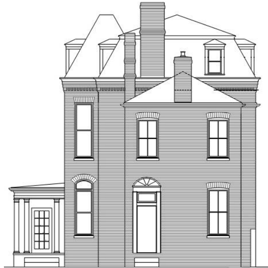
Photo 2: Proposed north elevation with chimney extension.
