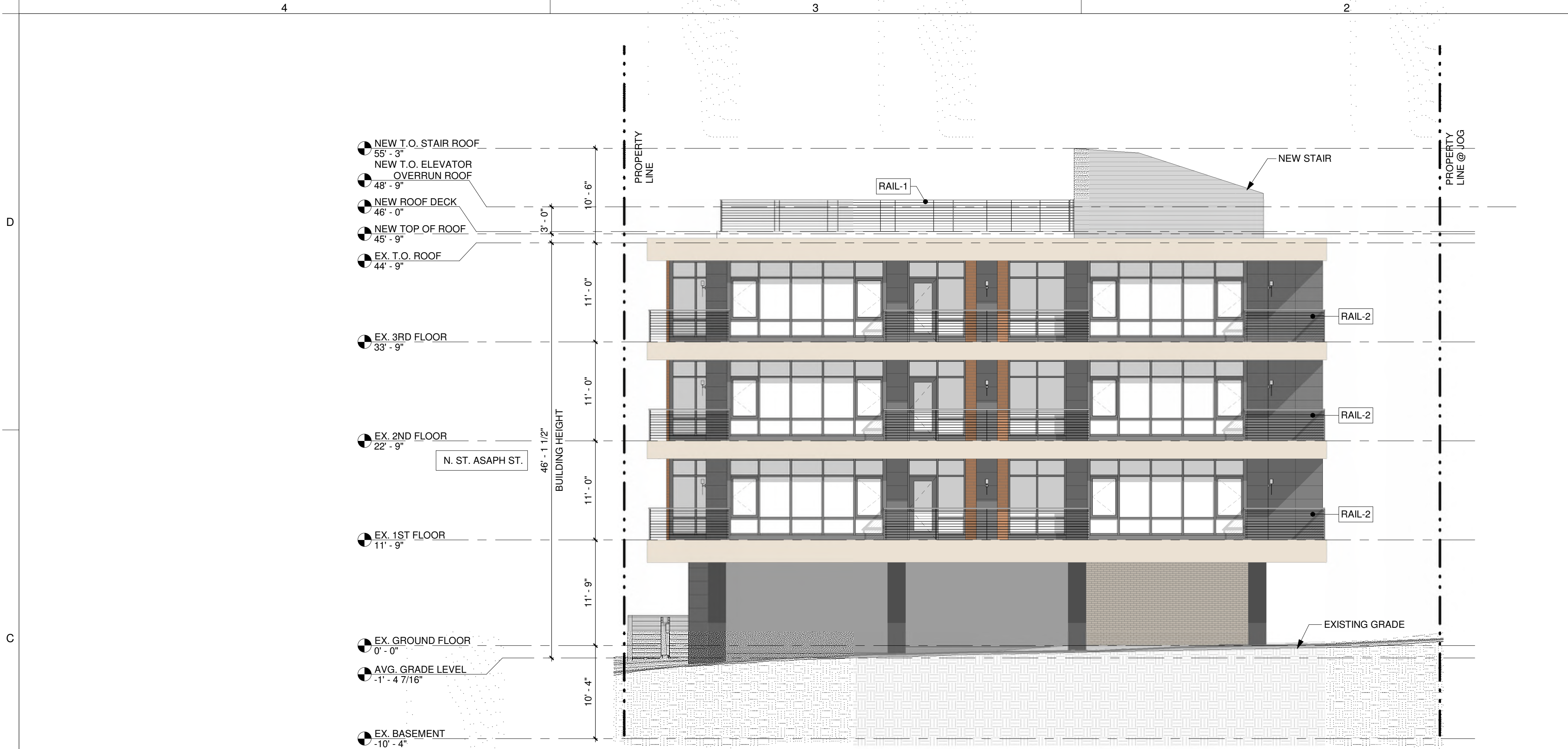
1 BUILDING ELEVATION - NORTH SCALE: 1/8" = 1'-0"
