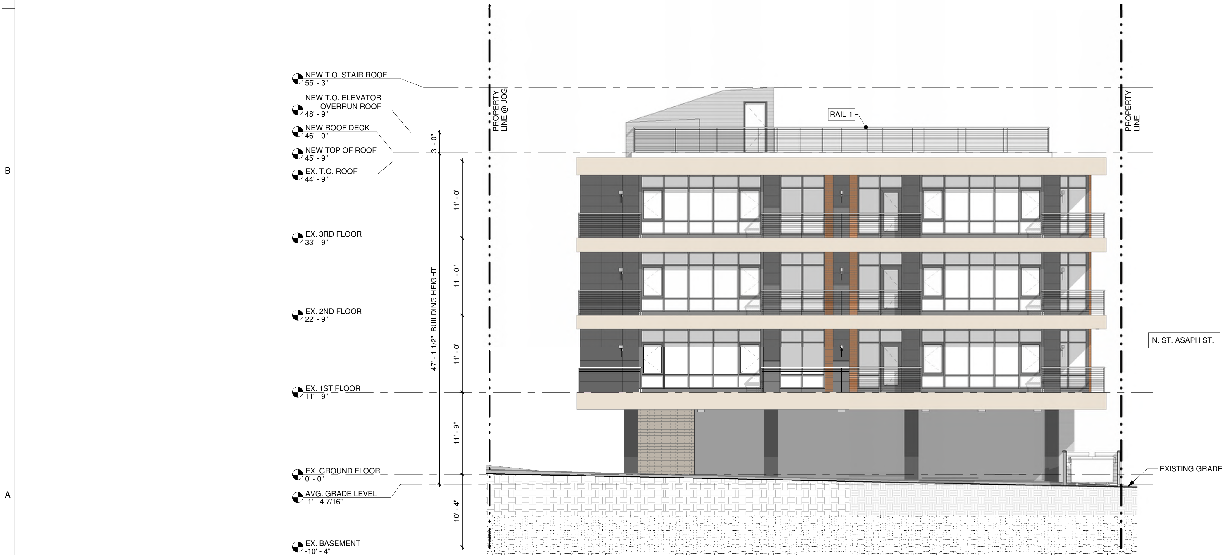
2 BUILDING ELEVATION - SOUTH SCALE: 1/8" = 1'-0"
