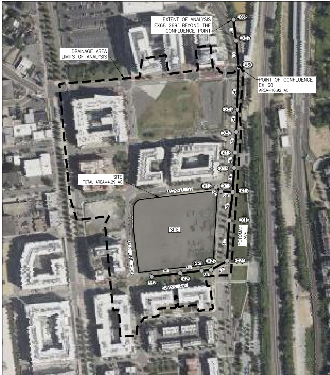
STORM SEWER OUTFALL ANALYSIS MAP SCALE: 1"=100'
