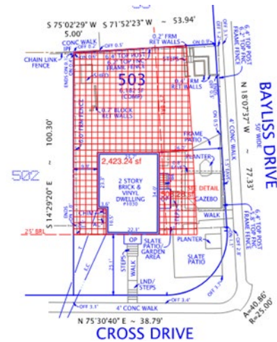
Figure 4: Area that can be enclosed with a 6.00-foot fence by right shown shaded
