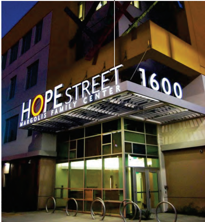
Face Illuminated Channel Letters Mounted on structural architectural rail
