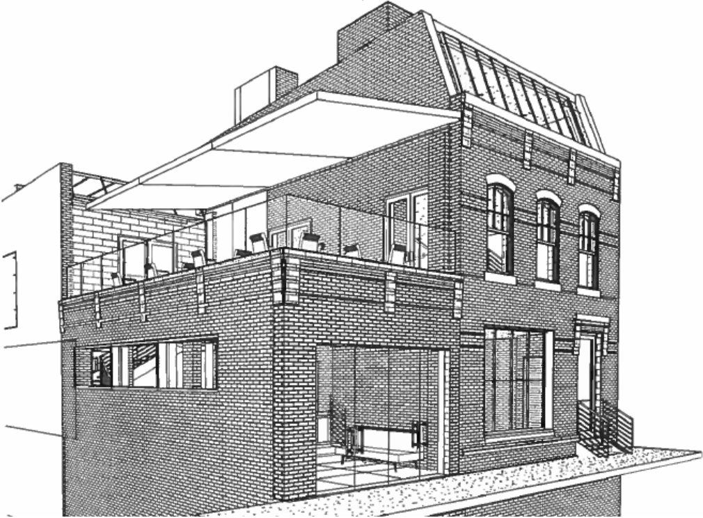
Figure 2. Perspective view of proposed addition and alterations to provide a second story terrace for outdoor dining with a retractable awning.
