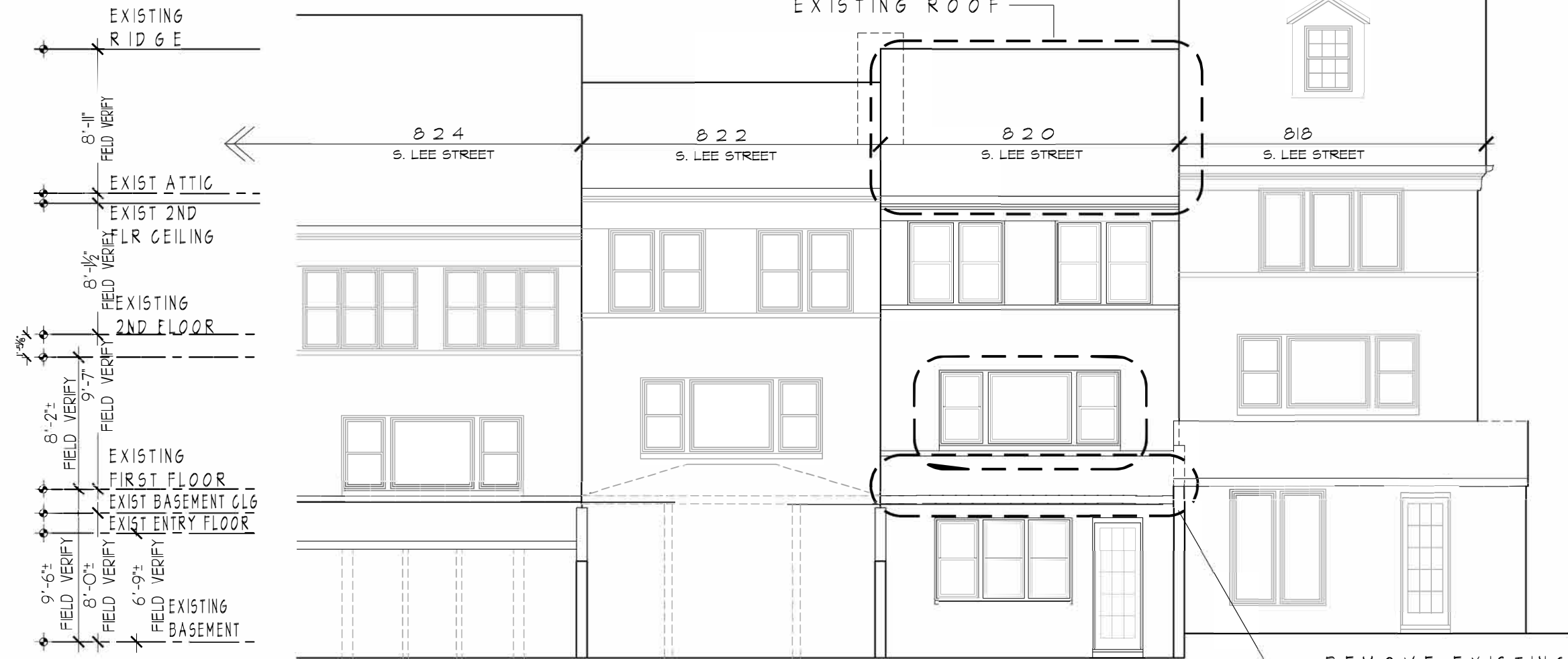
(C) EXISTING REAR SOUTH ELEVATION 1/8"=1'-0"
