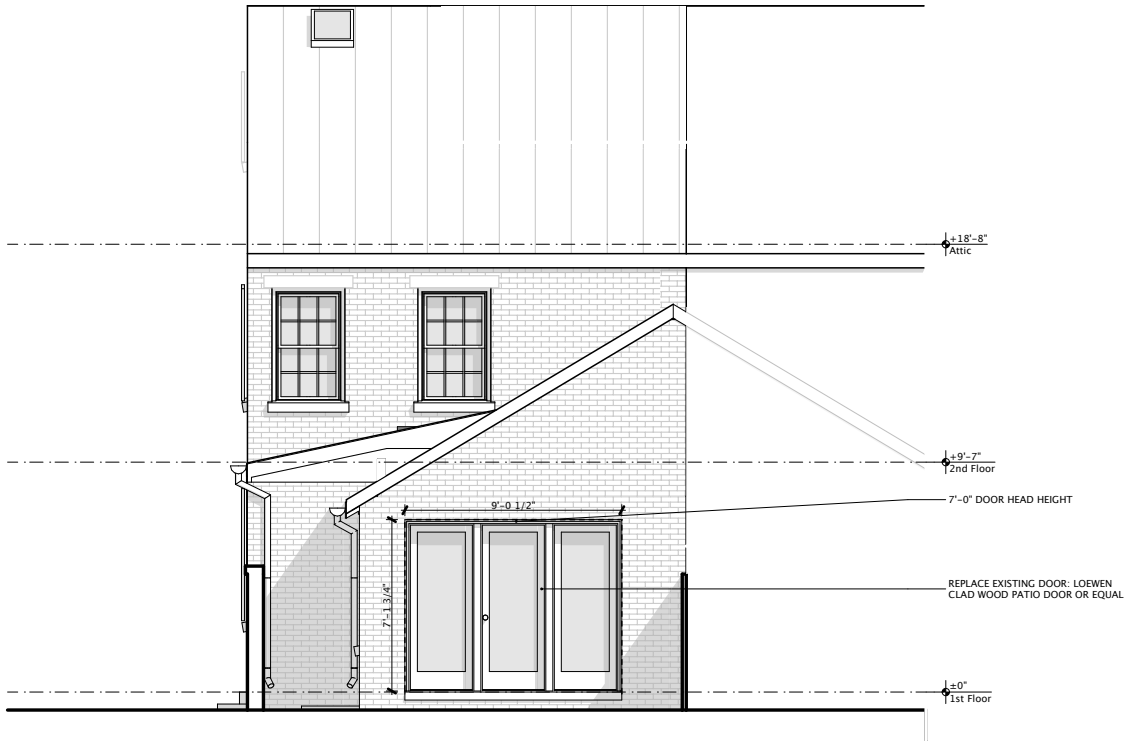
Proposed Rear (North) Elevation SCALE: 1/8" = 1'-0"
