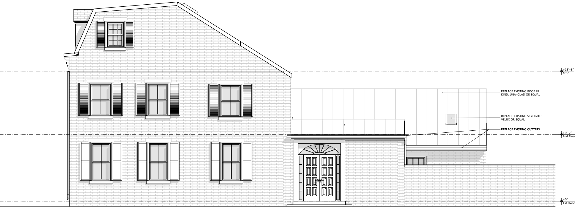
Existing Right (East) Elevation SCALE: 1/8" = 1'-0"
