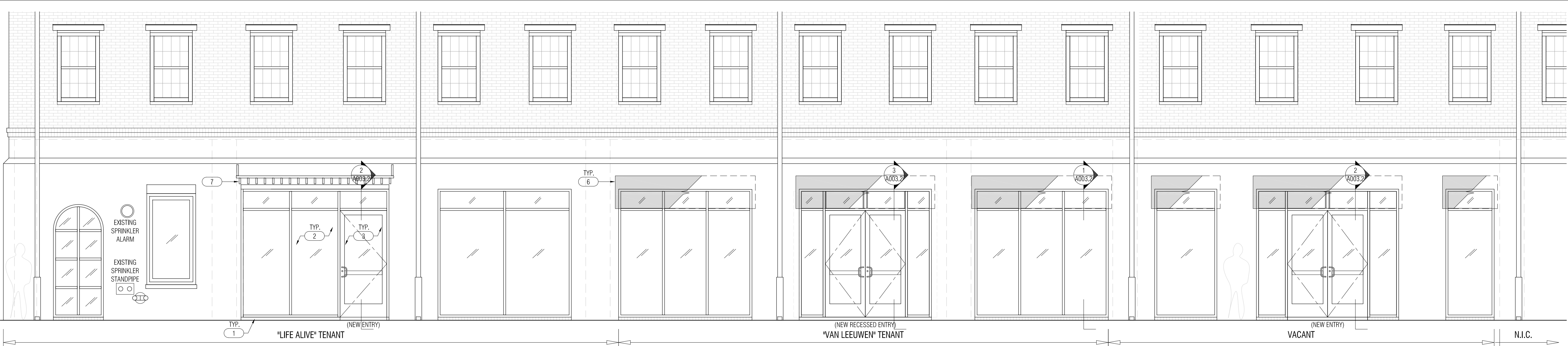
1 ELEVATION: KING STREET FACADE - NEW STOREFRONTS SCALE: 1/4"=1'-0"
