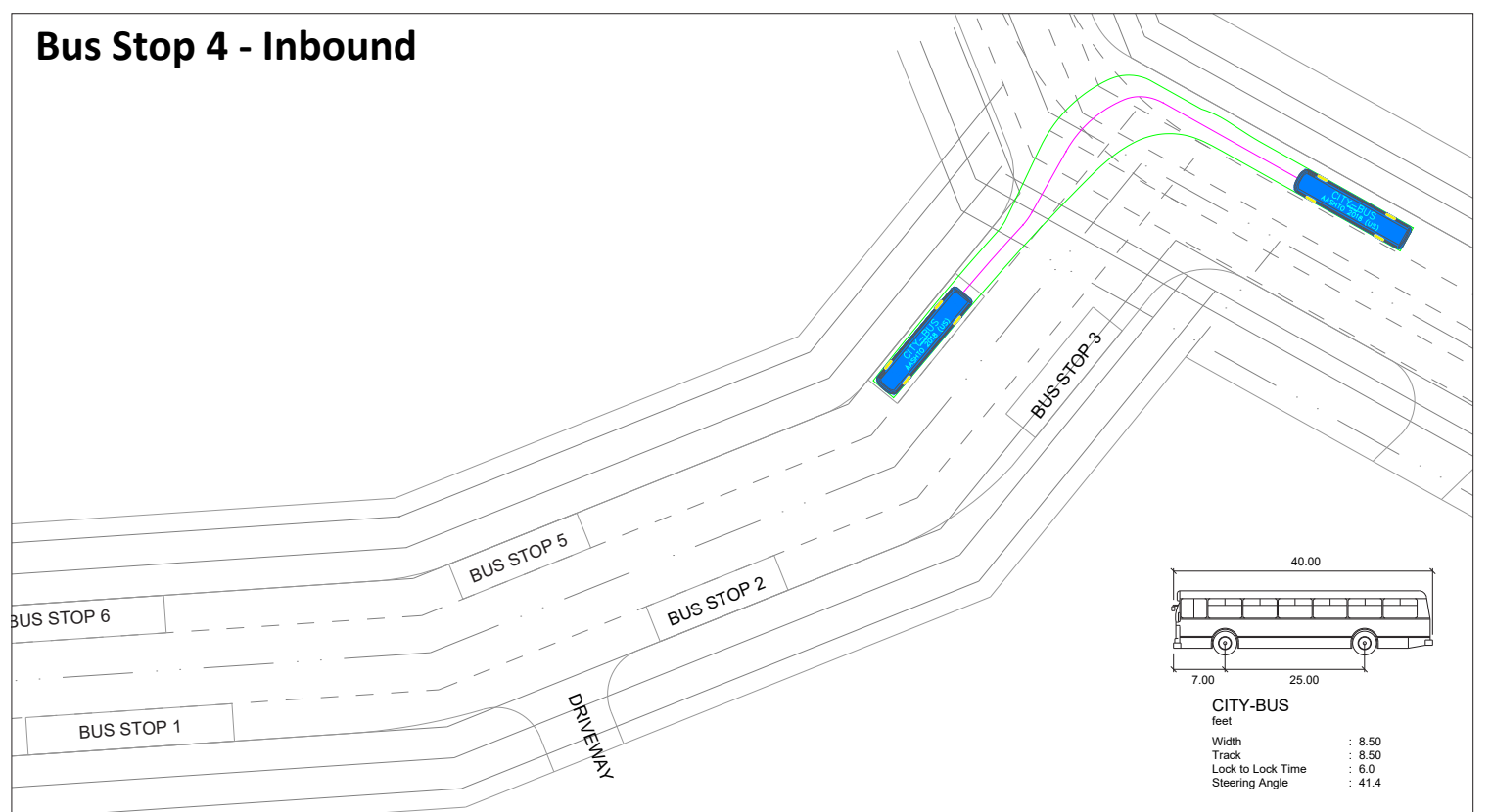
1 ENLARGED PLAN - TRANSIT HUB 10B SCALE: 1" = 30'-0"
