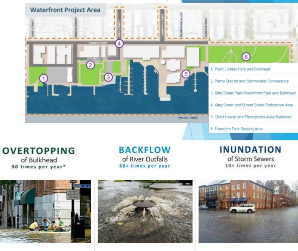
Requires raised bulkhead or other taller flood barrier(s). Requires riverine backflow prevention for storm sewer system. Requires larger storm sewer pipes, underground storage, and pumping.
