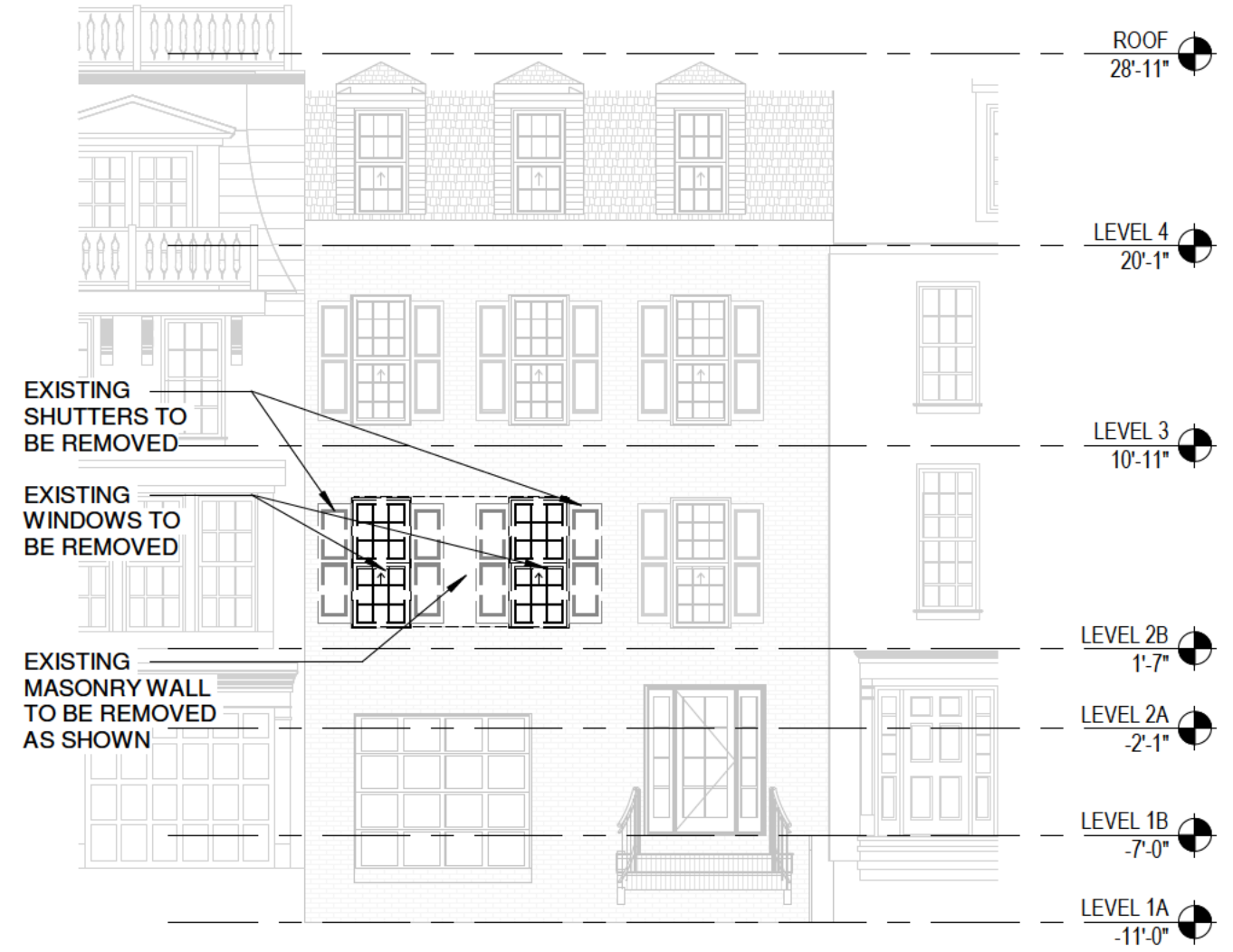
EAST (FRONT) DEMOLITION ELEVATION 1 1/8" = 1'-0" A02
