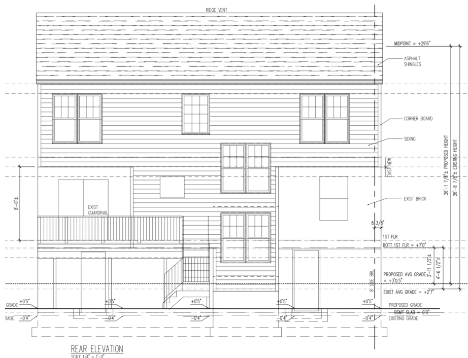
Figure 4: Rear elevation of proposed addition
