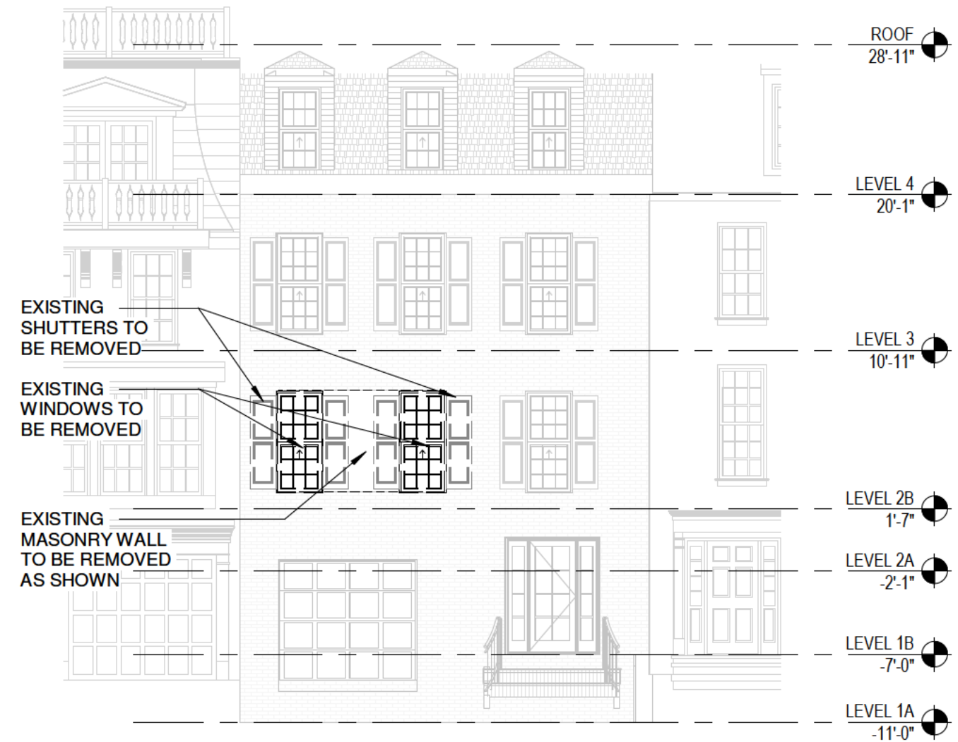
EAST (FRONT) DEMOLITION ELEVATION 1 1/8" = 1'-0" A02
