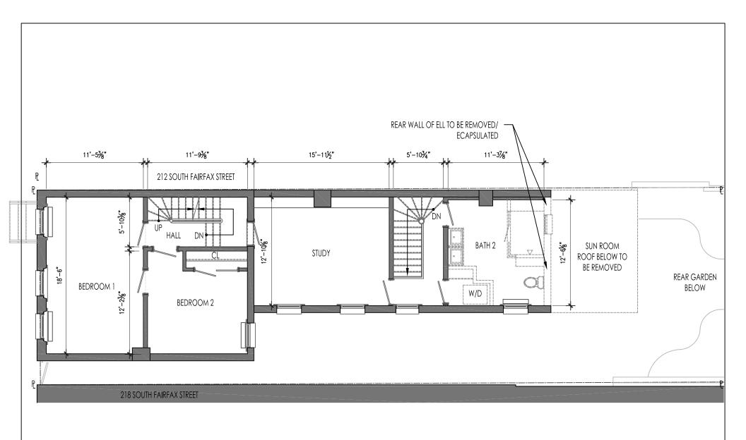
EXISTING 2ND FLOOR SHOWING PROPOSED DEMOLITION
