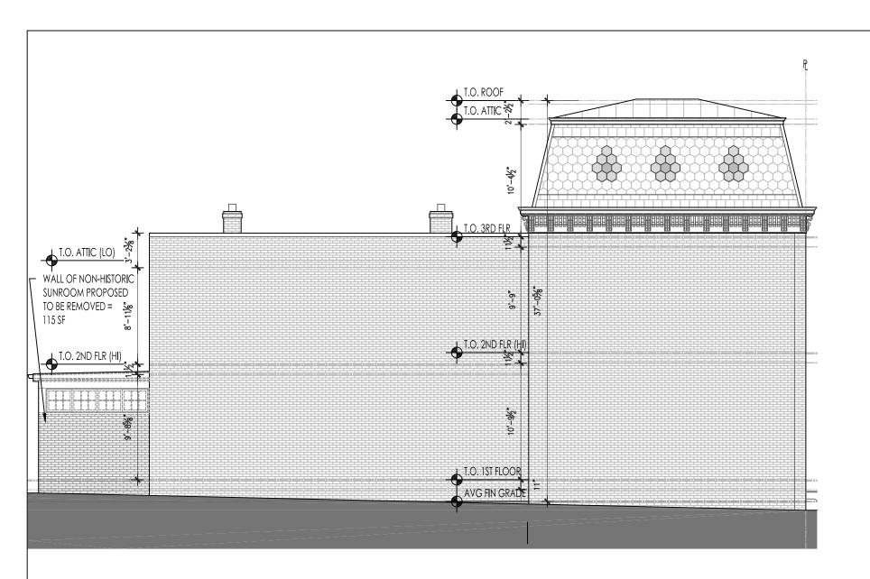
EXISTING NORTH SIDE ELEVATION SHOWING PROPOSED DEMOLITION
