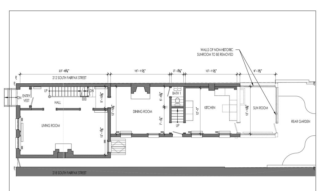
EXISTING 1ST FLOOR SHOWING PROPOSED DEMOLITION
