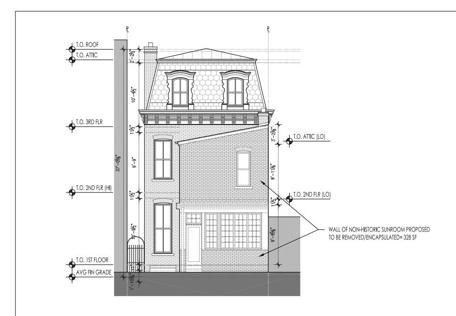
EXISTING REAR ELEVATION SHOWING PROPOSED DEMOLITION
