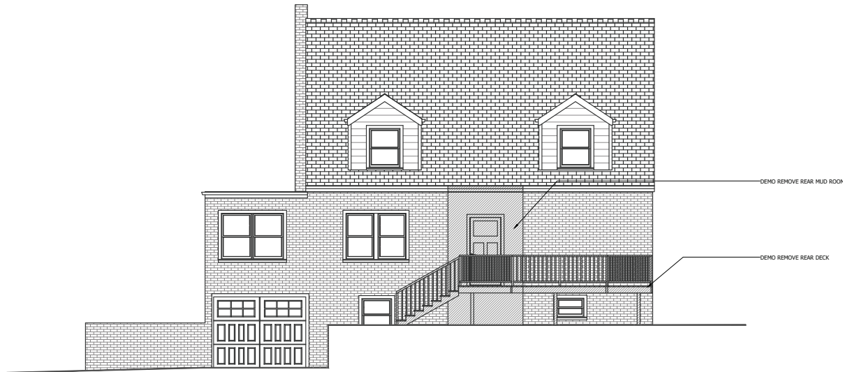
1) EXISTING DEMO REAR ELEVATION SCALE: 1/4" = 1'-0"
