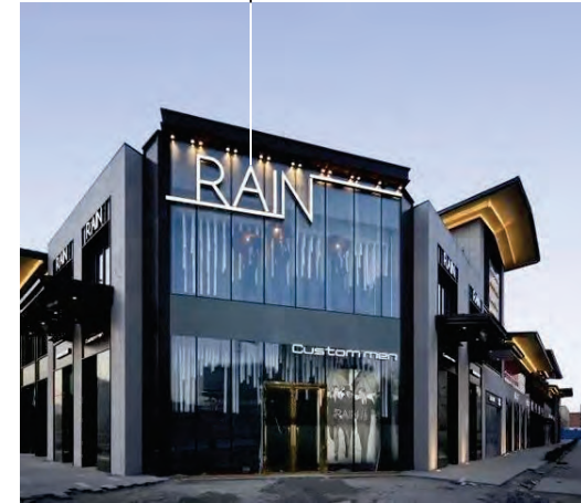
Face Illuminated Channel Letters Mounted to window glazing
