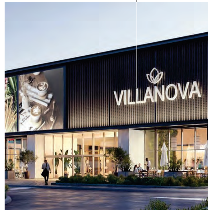
Fully Illuminated Channel Letters Mounted to facade metal tube cladding
