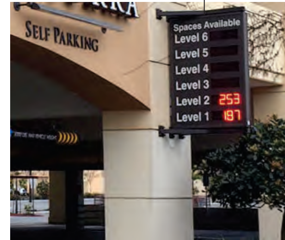
Smart Parking LED Entrance Signage
